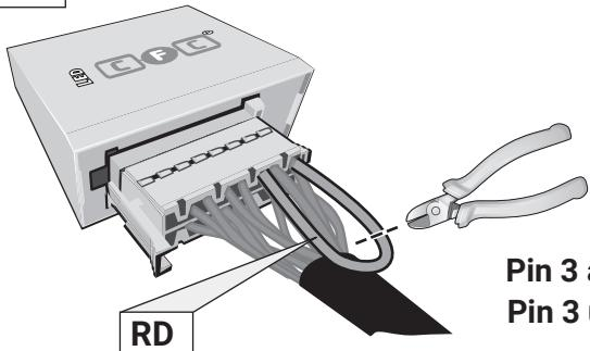
Pin 3 and Pin 2 disconnected
